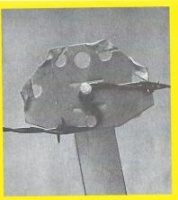
Keep turning until the wire reaches desired tension. An out-turned flange holds it securely in place.
