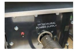
The first step is to connect the two umbilical cords provided between the Power Sources and Reference DAC. To insert the connector, set the slide lock to 12am.
