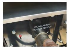
Then push the connector toward the unit and rotate clockwise until a locking sound is heard.
