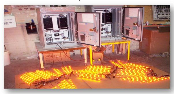
The Master Controller Power Modules, contain custom pulse width Power Modules which takes any power from 90VAC – 220VAC and turns it into the correct low power series circuit voltage, suitable for LEDline® units. There are VDC and other types of power supplies, which vary with application. (Please contact HIL-Tech Ltd. for details).
