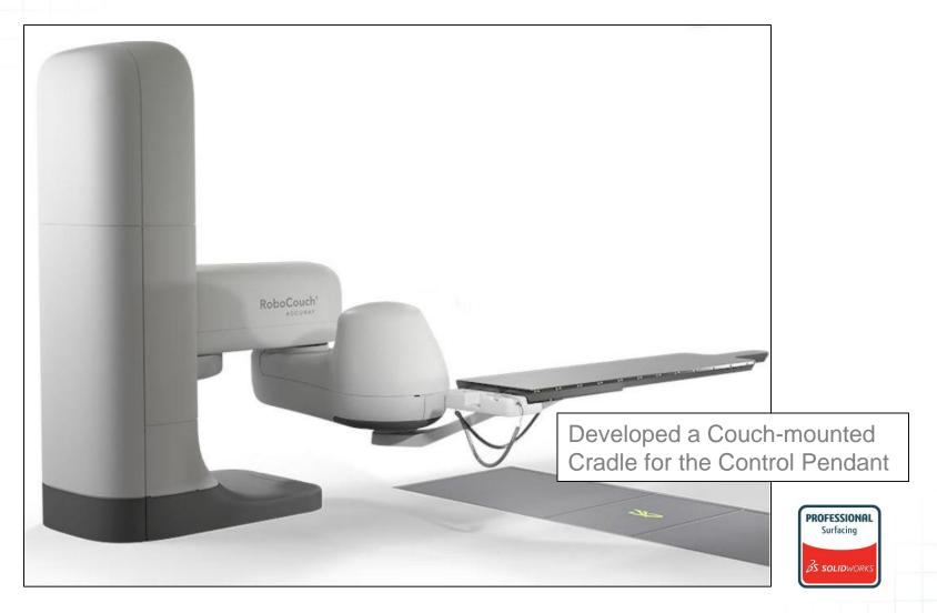
As part of the client's development team, designed and installed the large enclosures for the RoboCouch Patient Positioning System.
