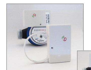
Client was using off-the-shelf enclosures for their wireless utility monitoring devices. Designed new enclosures around their existing PCBA's to enable product-specific new features and a custom corporate "look". Snap-together assembly minimizes the cost of US final assembly.
