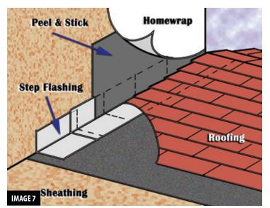
The peel-and-stick flashing adds another layer of protection by sealing over the step flashing onto the sheathing. If any water gets behind the housewrap, it will run onto the peel-and-stick flashing to daylight.
