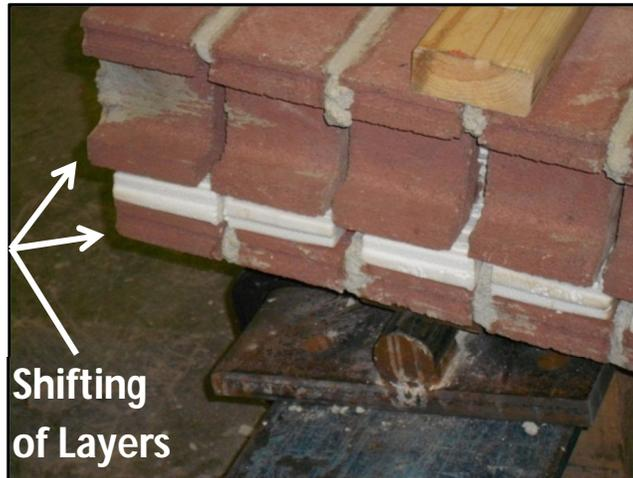
**Figure 16 – Wall 2 After Load is Released (Showing Shifting of Layers)**
