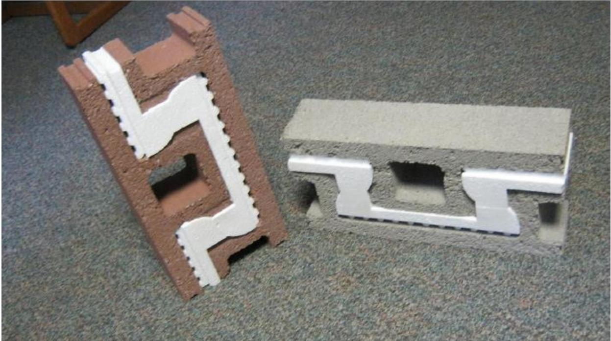
**COMPARISON OF CALCULATED DESIGN STRENGTHS TO LABORATORY TESTING RESULTS OF 8-INCH NRG CONTINUOUSLY INSULATED CONCRETE MASONRY UNITS (CICMU)**
