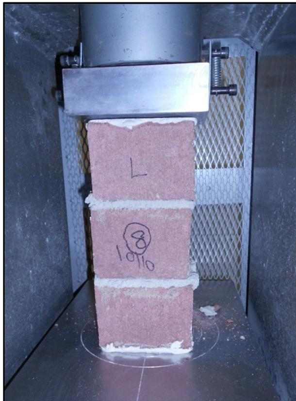
**Figure 6 – Prism Test Setup**
