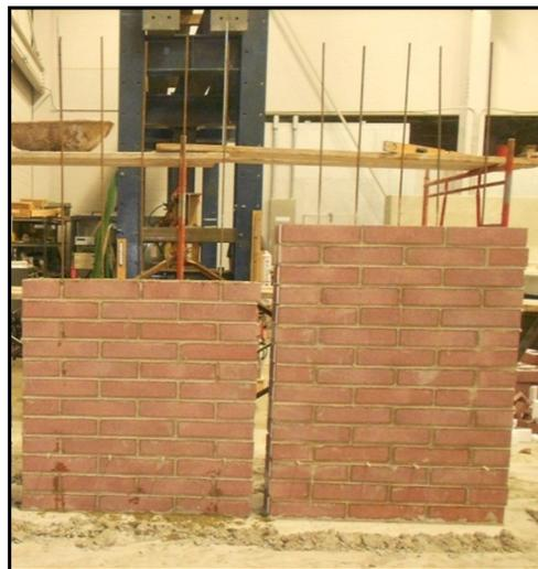
**Figure 10 – Wall Construction Showing Vertical Reinforcement**
