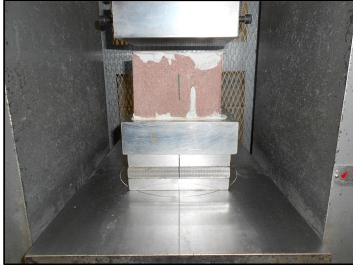
**Figure 4 – NRG Compression Test Setup for Individual Masonry Units**
