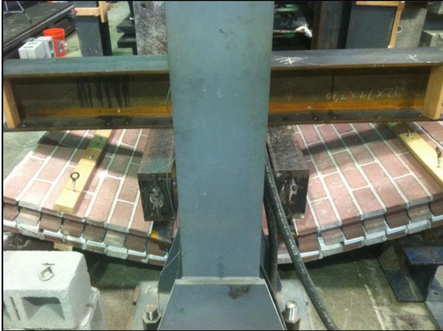
**Figure 14 – Wall 1 Under Maximum Deflection (Prior to Unloading)**
