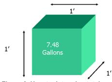
Figure 3. How to determine total volume in gallons
