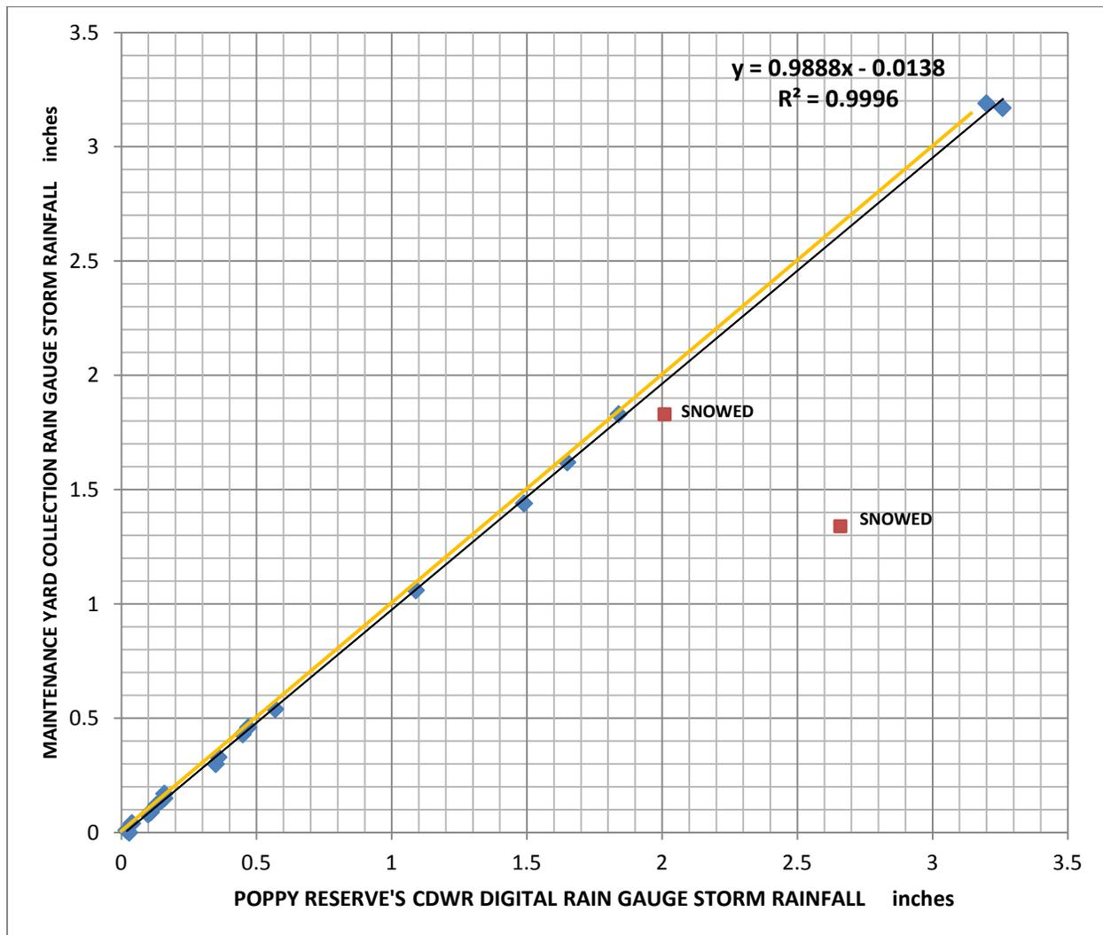
**FIGURE 1: MEASURED RAINFALL COMPARISON BETWEEN A CDWR DIGITAL RAIN GAUGE AND A CoCoRAHS COLLECTION RAIN GAUGE**
