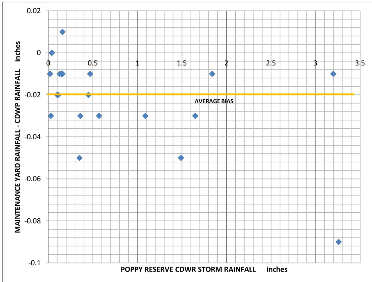
**FIGURE 2: DIFFERENCES IN MEASURED RAINFALL BETWEEN A CDWR DIGITAL RAIN GAUGE AND A CoCoRAHS COLLECTION RAIN GAUGE**
