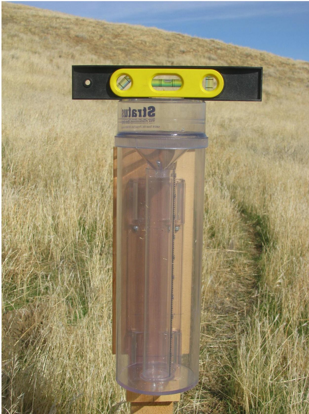
**FIGURE 3: CoCoRAHS STYLE RAIN GAUGE INSTALLED AT THE POPPY RESERVE**
