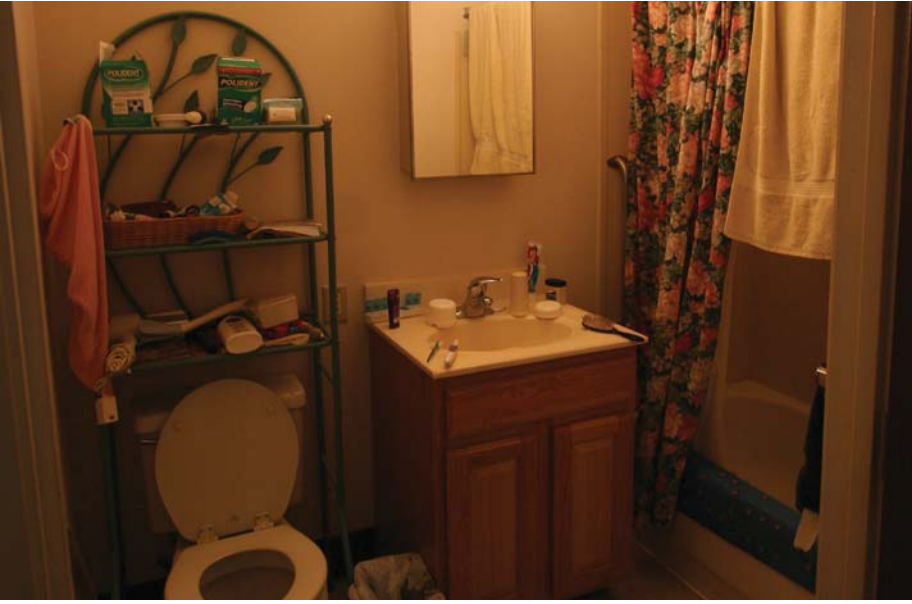
6. Bathrooms are dated but larger than minimal size. They do not have natural light and back up to the central corridor. Expansion of bathrooms to meet MAAB requirements would be difficult. Apartments do not have laundry hook-ups; there is a common laundry room on each floor.
