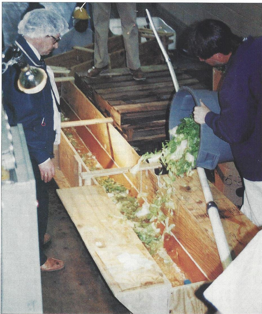
Vegetable waste is dumped into a prototype flume to test hydraulic behavior.
