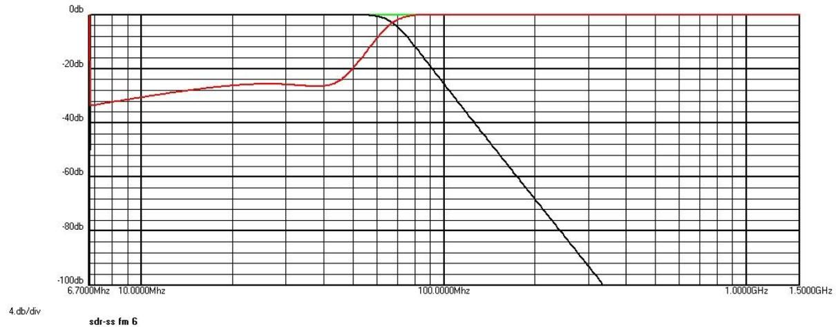
**Frequency response of the low pass filter L1, L3 = .16 uH, L2 = .257 Uh for 6 meters**
