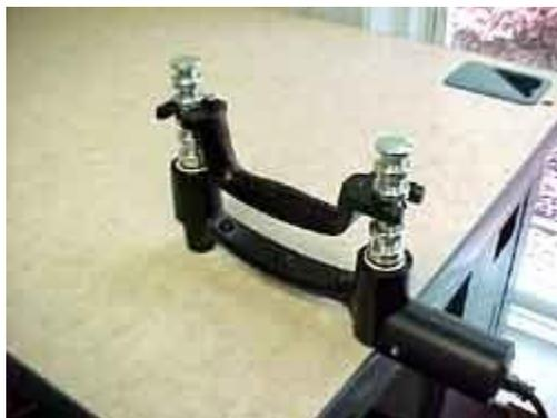
Method 2: Adjust the grip handle to position 4 (second from the widest). Insert the posts of the Hand Dynamometer into two 2-1/2 pound weights placed on the floor (back of dynamometer is pointing up) as shown. The sole purpose of the weights is to hold the Dynamometer in position for calibration.
