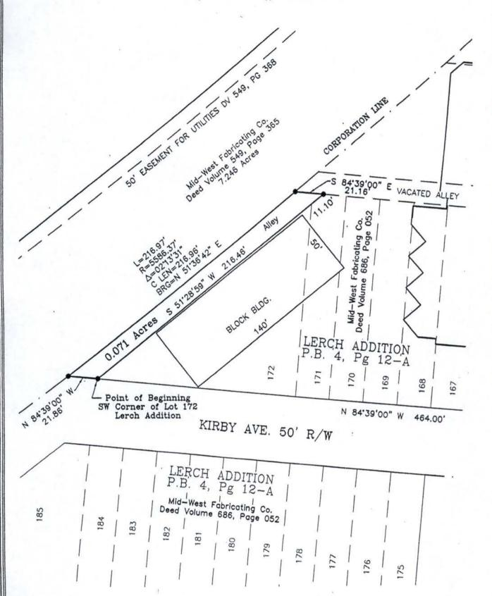
Bearings are based on an assumed meridian and are used to denote angles only. Bearings/Distances in parentheses are from previous deeds and/or surveys. FEMA Community Panel No. 390158 0175 D, Zone C.
