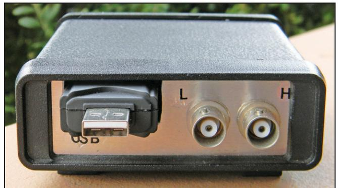
Figure 4 — Back view shows the USB and antenna connections.
