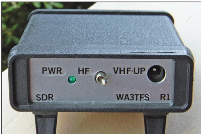
Figure 3 — Front view shows the HF and VHF-UP band switch.
