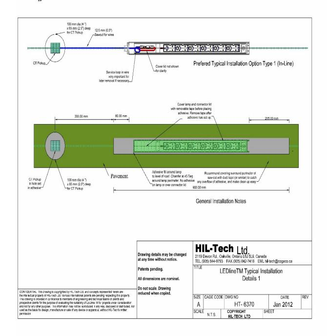
Typical saw cut depths for the lights and induction power distribution cables: **Please Note**; the induction power cables can also be separated from the lamps, please see the more comprehensive details in our standard Instillation guidelines.
