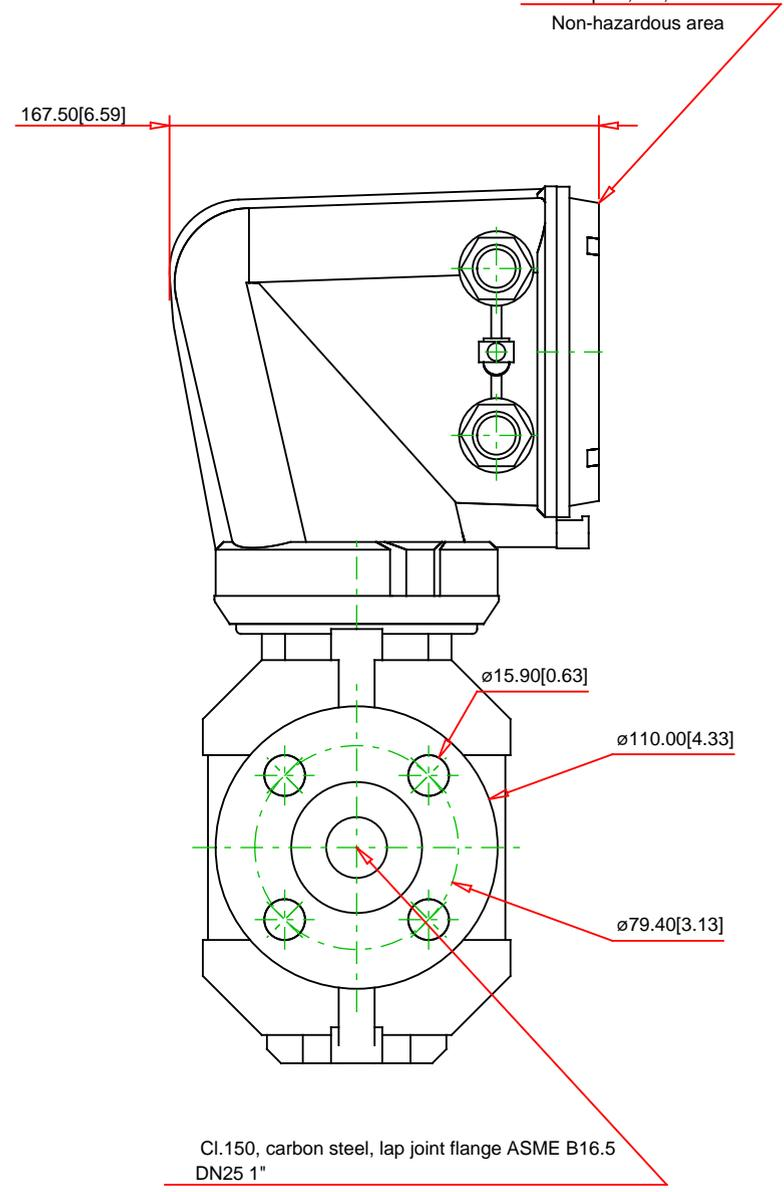
Cl.150, carbon steel, lap joint flange ASME B16.5
