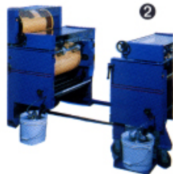
For ease in changing type and servicing, the second bottom printing station can be easily separated.
