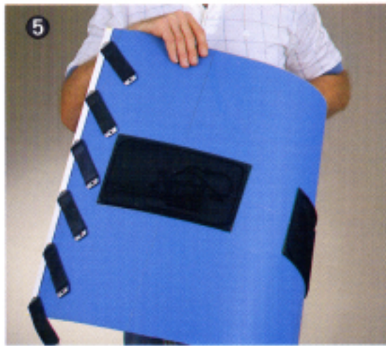
Flexback Printing Cylinder: Printing dies are mounted on quick change flexible plastic sheets, which are then wrapped around the printing cylinder and retained with rubber attachment bands. Recommended for those applications where large amounts of copy are being printed. Flexback sheets shown with rubber straps used to attach sheet to printing cylinder.
