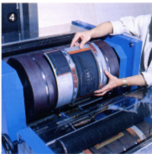
Magnetic Printing Cylinder: Uses curved metal type plates with permanently-mounted printing dies and/or channels for Kiwi Channelok type or baselock type. Recommended when frequent message changes are required.
