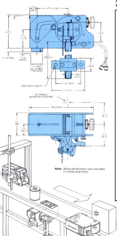
**Speed:** Up to 150 imprints/min. Maximum surface speed (webs or containers): 150 ft./min. (45.7 m/min.). (Actual production rate dependent upon sensor used. Consult factory for recommended rates.)
