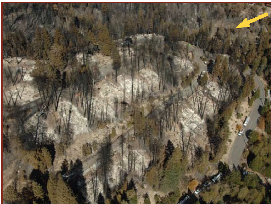
Figure 17. An aerial view of home destruction on Modoc Ln. (middle) and Inyo Ct. (top). Trinity Dr. is the road to the right (northeast) that wraps around the hill. Unconsumed tree canopies surround the home destruction. Burned canopies are over and between the destroyed homes. This indicates that the trees burned due to the burning homes, and the head fire that impacted Trinity Dr. from the north (arrow) did not continue into the subdivision. In this area, home destruction is primarily house-to-house. (Photo by Tom Iraci)
