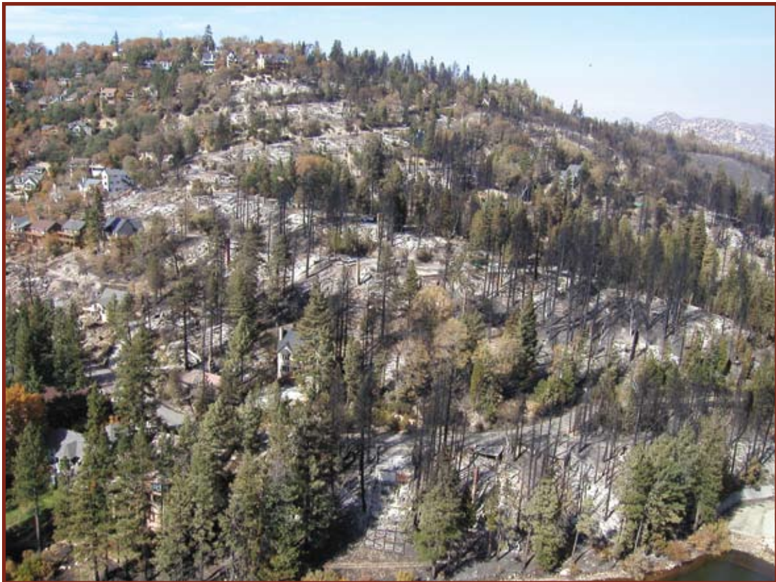
Figure 27. Aerial view to the northwest of homes on Brentwood Dr. (bottom) and Modoc Ln. (center). Areas with blackened trees are a result of the homes burning the vegetation. At about 1100, the wind shifted north-northwesterly, spreading fire and firebrands downhill to the southeast.
